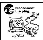
If foreign objects (metal fragments, water, liquids) enter the machines, first turn off the power switches and disconnect the power cord plugs from the outlet, and then contact your authorised TOSHIBA TEC representative for assistance. Continued use of the machine in that condition may cause **fire** or **electric shock**.
